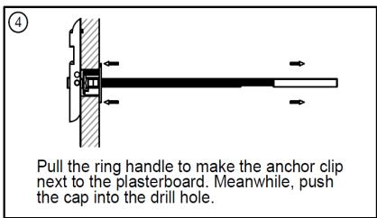
Pull the ring handle to make the anchor clip next to the plasterboard. Meanwhile, push the cap into the drill hole.
