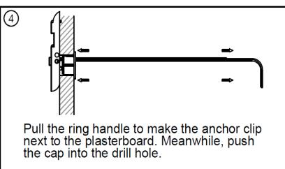
Pull the ring handle to make the anchor clip next to the plasterboard. Meanwhile, push the cap into the drill hole.
