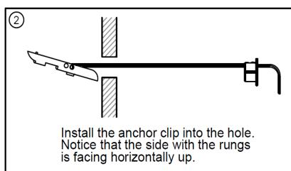
Install the anchor clip into the hole. Notice that the side with the rungs is facing horizontally up.
