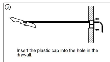
Insert the plastic cap into the hole in the drywall.
