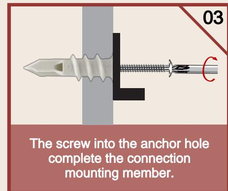
The screw into the anchor hole complete the connection mounting member.
