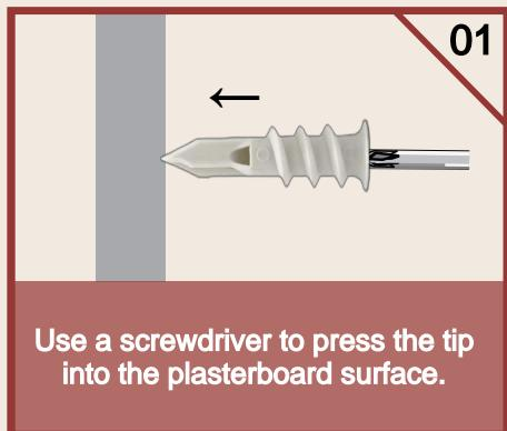
Use a screwdriver to press the tip into the plasterboard surface.
