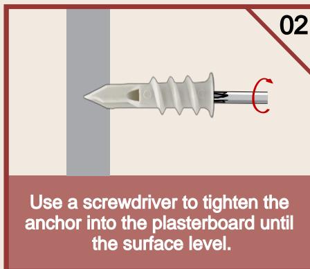
Use a screwdriver to tighten the anchor into the plasterboard until the surface level.
