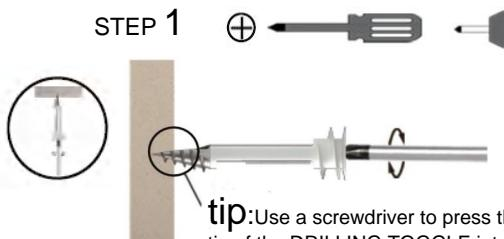
**tip:** Use a screwdriver to press the metal
