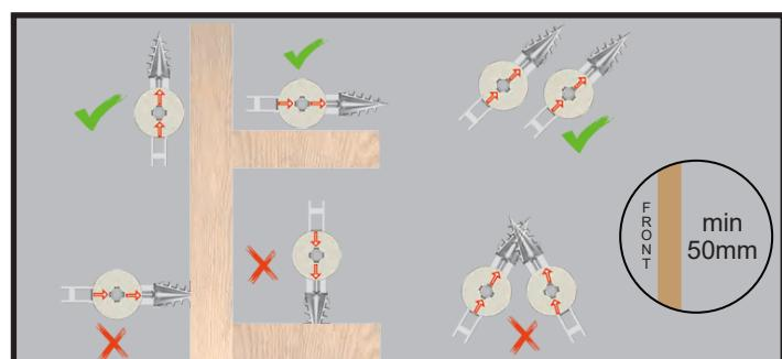
The arrows on the ZSM4B's white head indicate the metal part's direction behind the gypsum board. Align the arrow parallel to the wood strip to avoid it. For closely positioned toggles, ensure arrows are parallel. Use hand screwdrivers for fine-tuning alignment.
