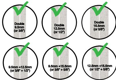
★ Specially designed for double layer plasterboards, with a thickness of 20-31mm.
