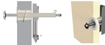
Anchoring into Plasterboards.
